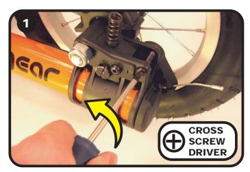
Remove the cross head screw from the front wheel lock assembly. Leave the 5MM lock nut seated in the assembly housing on the opposite side.
