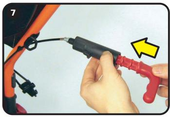
Insert the new brake handle into the brake cylinder. Push any excess cable back inside the cable housing.
