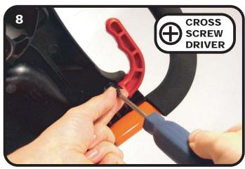
Reinstall the two screws that hold the brake and brake cylinder assembly to the bottom of the tray.
