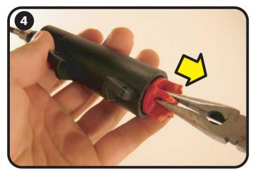
Using needle nose or similar pliers, remove the remaining portion of the Brake Handle from the Brake Cylinder.
