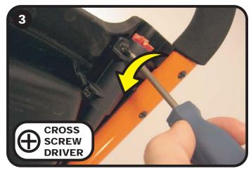
Unscrew the two screws that secure the Brake Cylinder to the under side of the tray.
