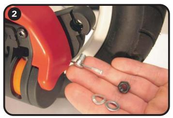
Remove the two washers and lock nut from the cable nut assembly. Leave the cable nut and protective cable end cap attached to the brake cable as shown.
