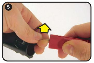
Pull the cable barrel end up and out of the brake handle.
