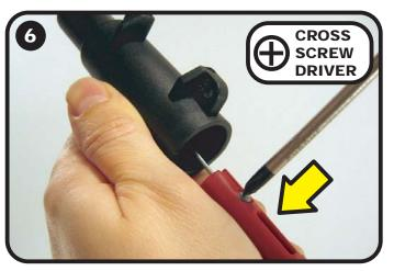
Install the new Brake Handle onto the cable. Carefully seat the cable end barrel into the handle using a small cross screw driver.
