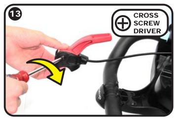
Assemble the Brake Lever on New Umbrella Brake Mount, push the end of the New Brake Cable Sheath and Brake Washer into it.
