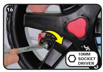
Tighten the cable lock nut while holding the brake hammer in the approximate position shown.
