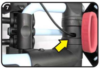
The New Brake Cable Sheath should pass through the bottom hole of Center Lower Hinge.
