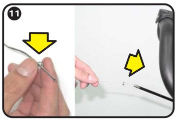
Put the Brake Washer to the New Cable from its end, then insert it to the New Brake Cable Sheath.
