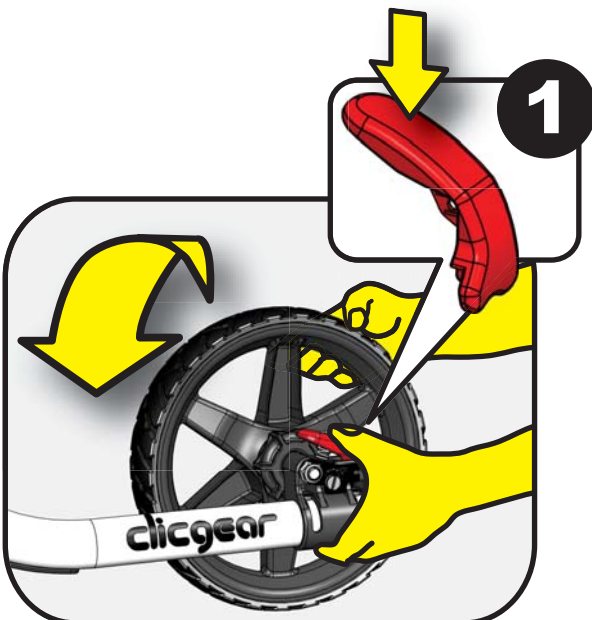
1 Squeeze the front wheel LOCK and rotate the front wheel to the horizontal position.
