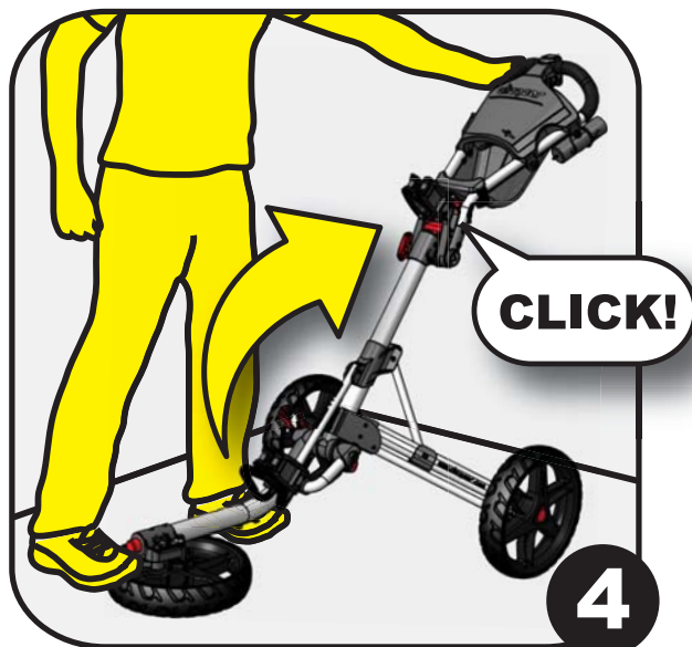
4 Extend the handle up and forward until the wheels extend and the handle CLICKS into place.
