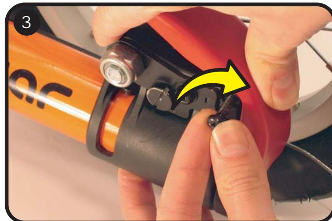
Insert the bolt while compressing the spring to align the holes. Begin threading the bolt into the locking nut on the opposite side, finger tight only.
