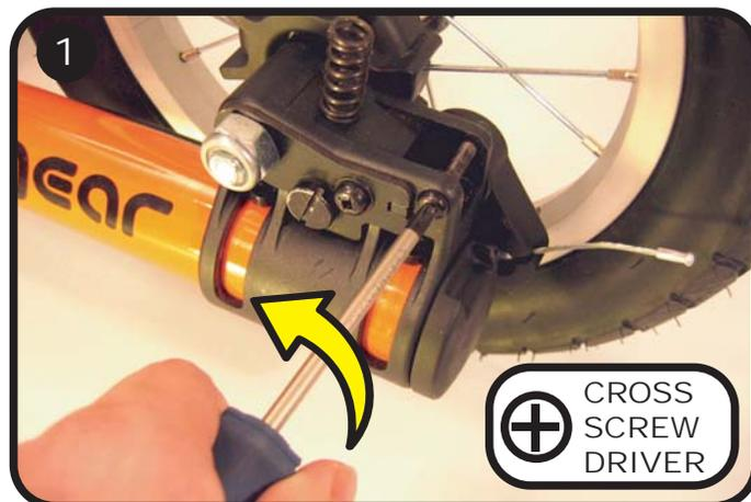
Remove the cross head screw from the front wheel lock assembly. Leave the 5MM lock nut seated in the assembly housing on the opposite side.
