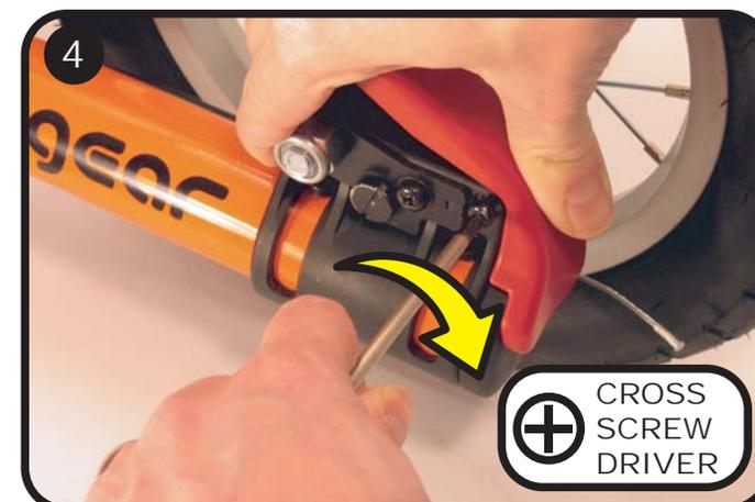
Tighten the bolt using a cross head screw driver. Do not over tighten the screw as it will interfere or limit the action of the front wheel lock.
