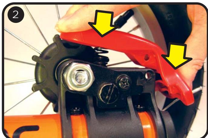
Install the new front wheel lock and ensure the spring is seated square to the handle. Push the handle down to compress the spring and align the bolt holes.
