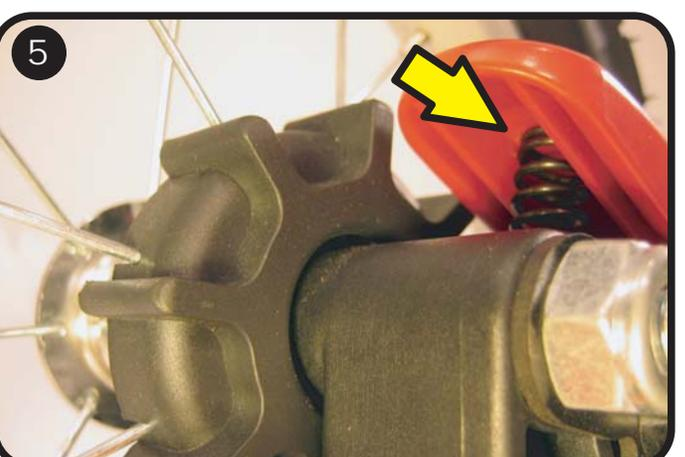
Check that the spring has remained seated square to the lock lever.
